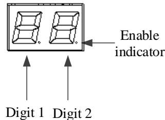
DP3C series displays running speed, state machine/operation mode, node address, alarm fault and other information through two-digit LED display.
